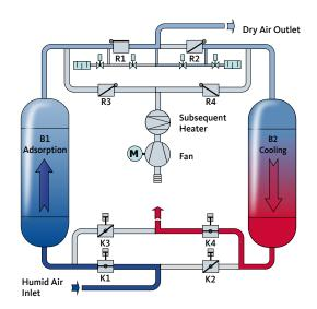
reached the same operating pressure. Cooling takes place in the opposite direction to adsorption from the top to the bottom.
